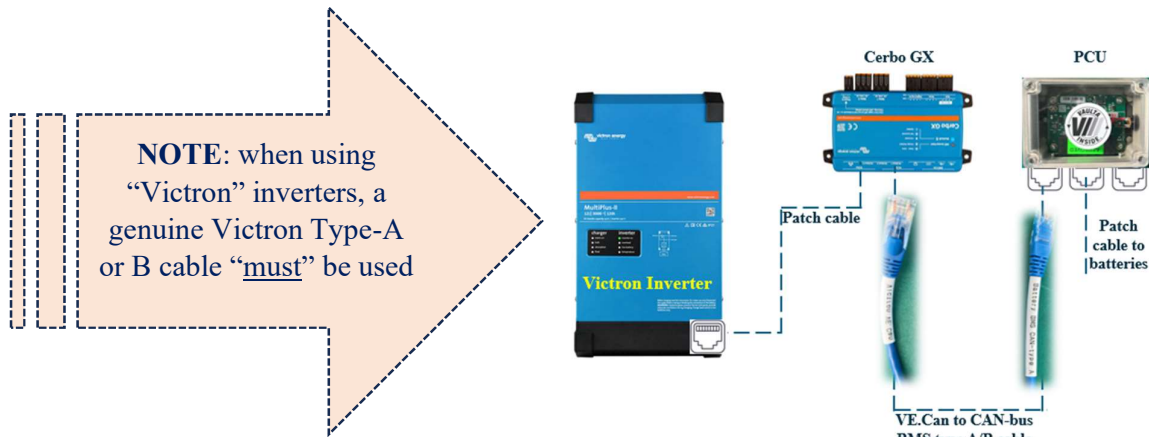
Fig 8. In the case of Victron inverters, PCU is connected to Cerbo GX gateway via genuine Victron path leads called “VE.Can to CAN-bus BMS type A or B”. All other COMMS cables are still standard patch leads
