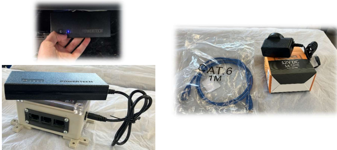
PCU and its UPS
